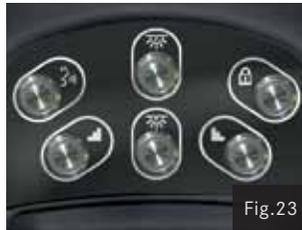
When activated the relevant button will illuminate on the control panel. The step will extend from its retracted position to its fully extended position (Fig. 24). The steps can be retracted by pressing the appropriate button for a second time. Each step will automatically retract when the parking brake is released.
