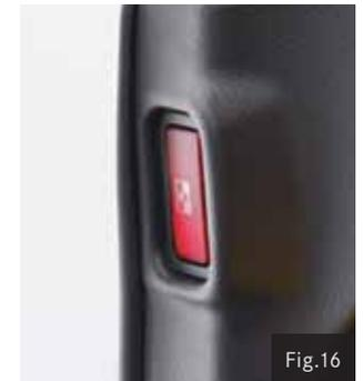
If partial lock is engaged and the driver has the brake pedal depressed, all doors are locked and the switch halo will remain on (not flashing) while full lock is engaged.
