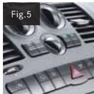
The driver can switch the heating in the rear compartment on and off by activating the rear heater control switch (Fig. 4). This enables the driver to have full control over the rear heating and ventilation system. The master control switch on the dashboard needs to be depressed (red light on) in order for the heater controls to fully function. (Fig. 5). In addition the driver can control the temperature and fan speed settings via the overhead heater control. (Fig. 6).
